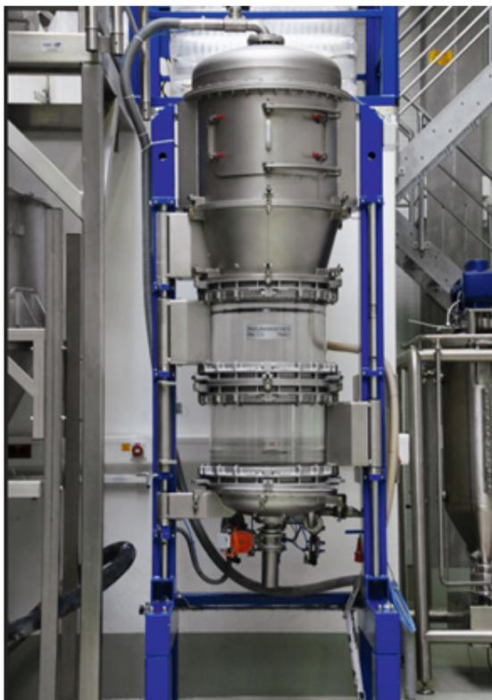
The Zeppelin Systems pneumatic mixer (homogenizing silo with fluidized bed bottom) produces a homogeneous mixture without mechanics, friction or high friction.
